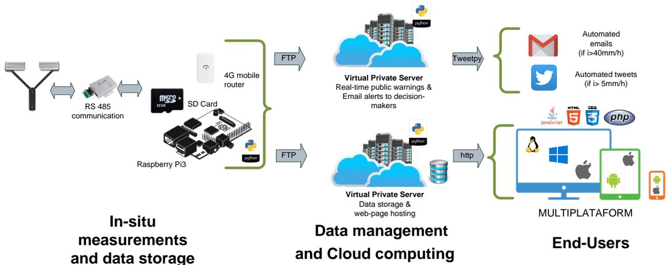
Figure 4. Visual representation of the architecture system.
