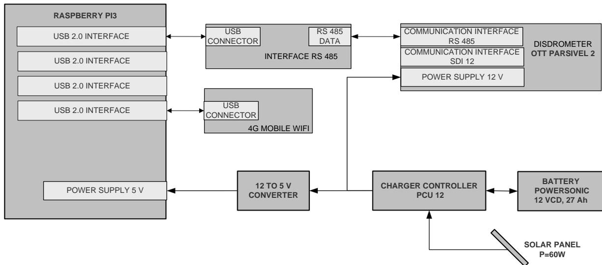
Figure 3. Block diagram of connections between components in each station.
