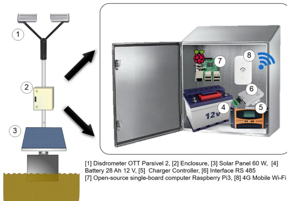
Figure 2. Main components of the system using cloud computing and real-time alerts through Twitter.
